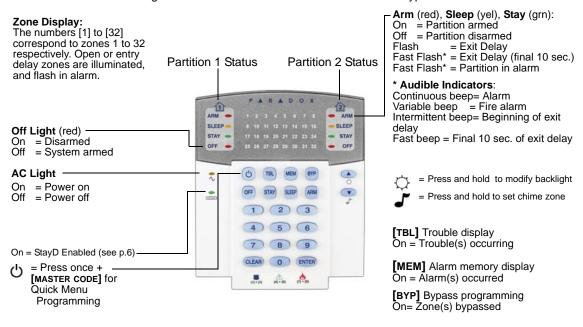
Figure 3: MG32LRF — 32-zone Wireless LED Keypad
