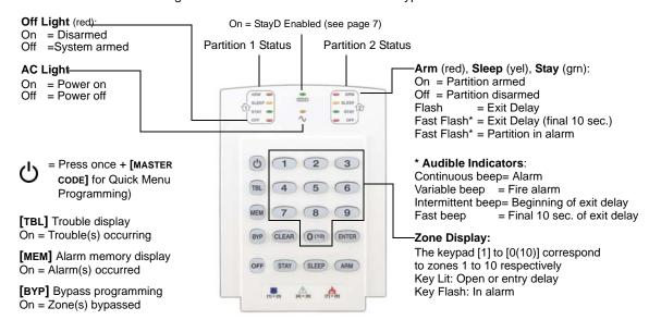
Figure 2: MG32LED —32-zone Hardwired LED Keypad
